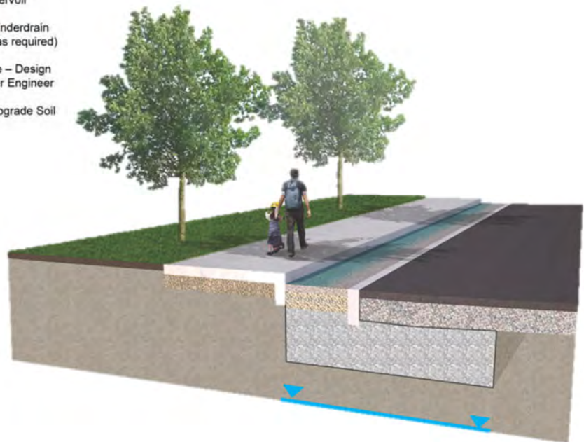
Figure 4-4. Examples of permeable pavement types (top) and use within the road right-of-way (bottom right)
