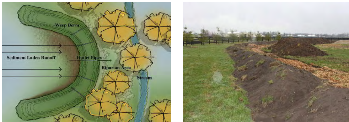
Figure 3-4. Schematic and example of a filter berm (Guffey, 2012)
