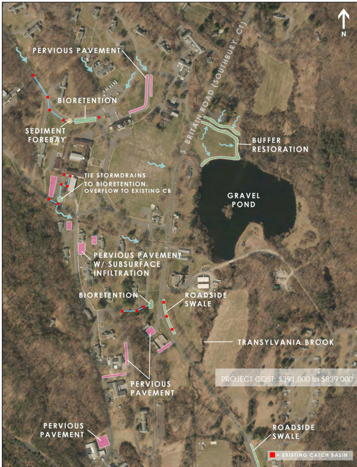
Figure 4-12. BMP Concept: State Facility 2
